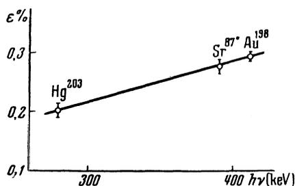
Fig. 1. The dependence of the efficiency of the gas discharging counter of the  $\gamma$ -quanta energy.
