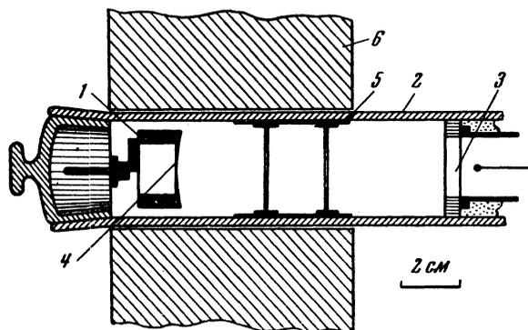
Fig. 2. Device for measuring the intensity of electrons. 1. Aluminum cup; 2. Vacuum tube; 3. Gas-discharging counter; 4. Source; 5. Aluminum diaphragm; 6. Electromagnet.
