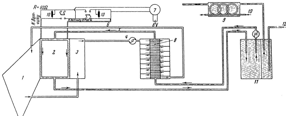
FIG. 3. Diagram of thermostatic regulation. 1— photographic camera body, 2— head of chamber, 3— illumination box, 4— air blower, 5— thermostatically-controlled water, 6— thermostatically-controlled air, 7— ratio meter, 8— radiator, 9— refrigerator, 10— compressed air for the expansion apparatus, 11— thermostatic bath, 12— tap water. The resistances are given in kilohms.
