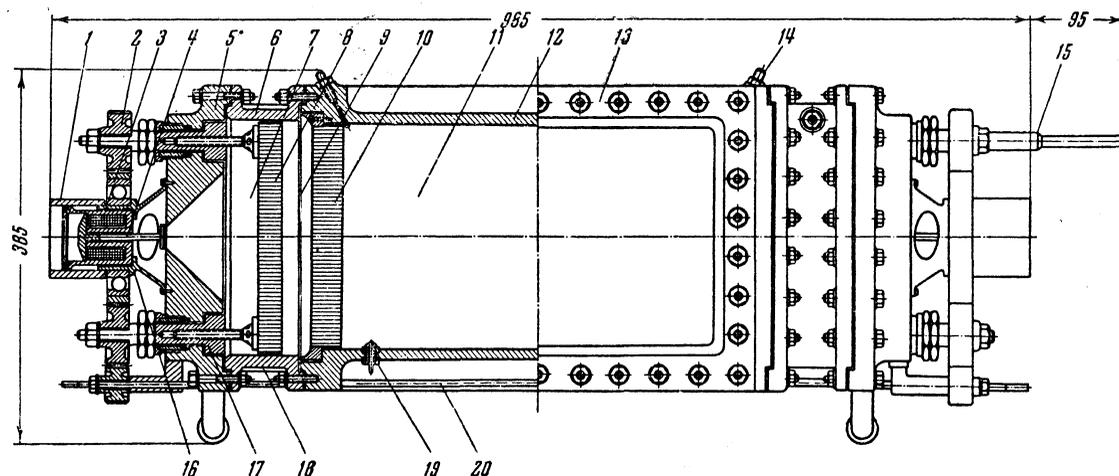
FIG. 1. Diagram of Chamber. 1- magnetic shield, 2- gears, 3- brass cylinder, 4- valve, 5- cover of expansion head, 6- case of expansion apparatus, 7- expansion apparatus, 8- movable grid, 9- rubber diaphragm, 10- stationary grid, 11- glass, 12- case of chamber, 13- flange, 14- fitting for filling the working volume, 15- vernier, 16- bushing for fastening valve, 17- mechanism for displacing movable grid, 18- water jacket, 19- input point for "clearing" field, 20- rod connecting the gear trains.
