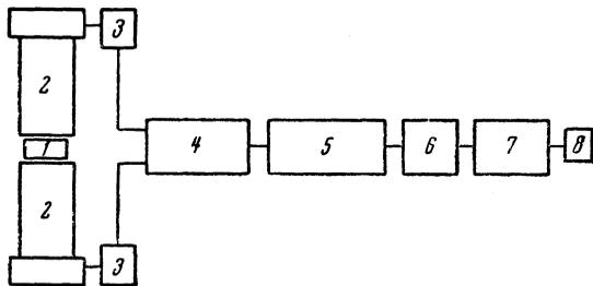
FIG. 2. Block diagram of the circuitry. 1 crystal; 2 PM-19; 3 cathode follower; 4 coincidence unit; 5 amplifier; 6 discriminator; 7 electronic counter; 8 mechanical counter.
