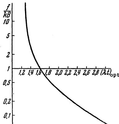
FIG. 3. Curve for determining the optimum length of time for observing the decay of  $C^{11}$
