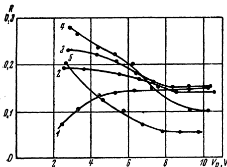
FIG. 6. The variation of the quantity R as a function of the energy of primary electrons for W and Ba-W with coverage corresponding to: 1- \Delta\varphi=0 (W); 2- \Delta\varphi=0.7 ; 3- \Delta\varphi=1.5 ; 4- \Delta\varphi=2.4 ; 5- \Delta\varphi=1.9 eV (Ba).
