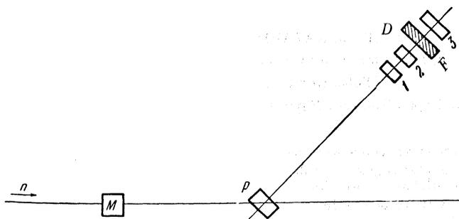
FIG. 1. Arrangement of the apparatus.  $n$  - neutron beam;  $P$  - scatterer;  $D$  - detector; 1, 2, 3 - scintillation counters;  $F$  - filter; monitor.
