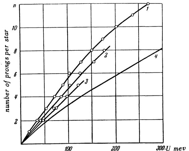
FIG. 5. Relation between number of black prongs per star and excitation energy of Ag and Br nuclei, for proton energies: 1-660 mev, 2-460 mev, 3-130 mev, 4-theoretical evaporation curve (Ref. 13).
