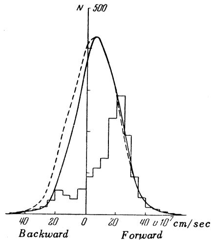
FIG. 2. Distribution of nuclei according to recoil velocity component  $v$ . The solid curve is the distribution corrected for unobservable cases, the dashed curve was calculated from formula (2) of the present paper.
