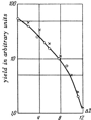
FIG. 7. Yield of nuclei with varying  $Z$  from bombardment of Ag and Br by 460 mev protons. The crosses are the results obtained in Ref. 14 and are adjusted to coincide with the present experiment at  $\Delta Z = 0$ . ( $\Delta Z = Z_{in} - Z_{final}$ ).
