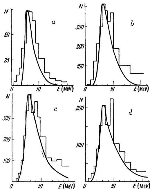
FIG. 9. Energy spectrum of protons for varying initial excitation energy of the nucleus. Computed evaporation spectra are shown for the following nuclear excitations: a) 0–50 mev ( $U_{av} = 25$  mev); b) 50–100 mev ( $U_{av} = 75$  mev); c) 100–150 mev ( $U_{av} = 125$  mev); d) 150–200 mev ( $U_{av} = 175$  mev).
