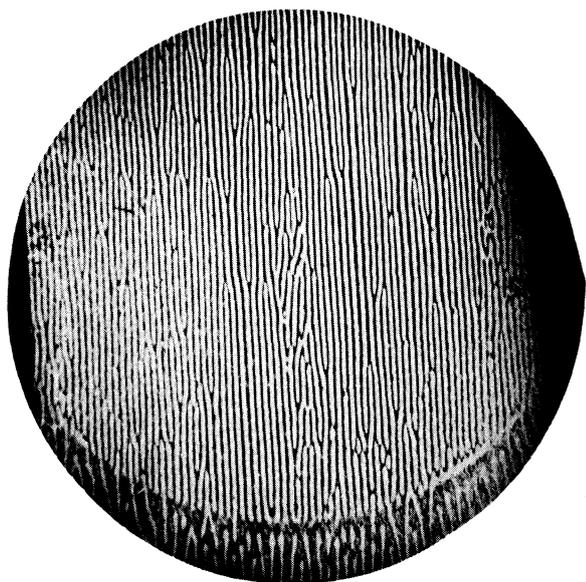
FIG. 3. View of the surface of the disc 50 mm in diameter (sample No. 1).  $T = 2.165^\circ \text{K}$ ,  $h = 0.950$ ;  $\eta = 0.62$ ,  $a = 0.54 \text{ mm}$ .
