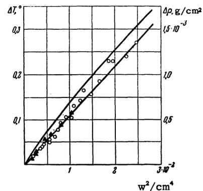
FIG. 3. Dependence of the density discontinuity  $\Delta\rho$  (lower curve), and the temperature discontinuity  $\Delta T$  computed from the change in density (upper curve), upon the square of the thermal current density. o) measurements in the 3-mm chamber; ▲) measurements in the 1.5-mm chamber.
