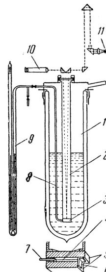
perature within the chamber began to rise, and, as it passed the  $\lambda$ -point, a visible boundary appeared within the chamber near the heater and moved toward the cold end. It could be maintained at any point in the chamber by suitable adjustment of the power or of the temperature of the external bath.
