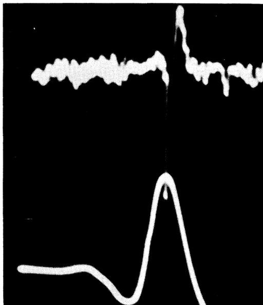
FIG. 2. Measurement of line position and width by means of a double beam oscillograph; lower beam-ferromagnetic resonance signal, upper beam-proton resonance signal in the same magnetic field.
