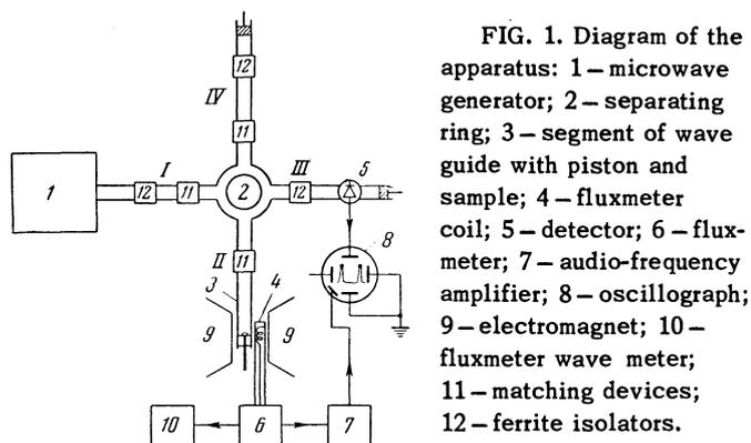
FIG. 1. Diagram of the apparatus: 1 – microwave generator; 2 – separating ring; 3 – segment of wave guide with piston and sample; 4 – fluxmeter coil; 5 – detector; 6 – fluxmeter; 7 – audio-frequency amplifier; 8 – oscillograph; 9 – electromagnet; 10 – fluxmeter wave meter; 11 – matching devices; 12 – ferrite isolators.
