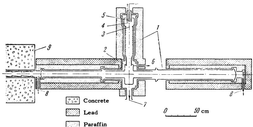
FIG. 1. Schematic diagram of the apparatus. 1 - apparatus shell, 2 - diaphragm, 3 - diaphragm with grid, 4 - spherical grid, 5 - proportional counter, 6 - high voltage electrode, 7 - diffusion pump outlet, 8 - monitors, 9 - reactor shield.
