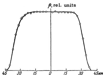
FIG. 3. Neutron density distribution over the beam diameter.
