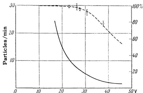
FIG. 2. Integral distribution of pulse amplitudes of  $H^+$  ions – dotted curve; dependence of the background on the discriminator level – solid curve;  $\circ$  – decay protons (control values).
