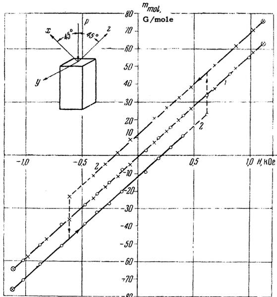
The dependence of molar magnetic moment on the size of the applied field: 1 – without pressure, 2 – pressure on specimen  $\sim 500 \text{ kg/cm}^2$ ; O – values obtained while changing the field from  $-1100$  oersteds to  $+1100$  oersteds x – while changing the field in the opposite direction.
