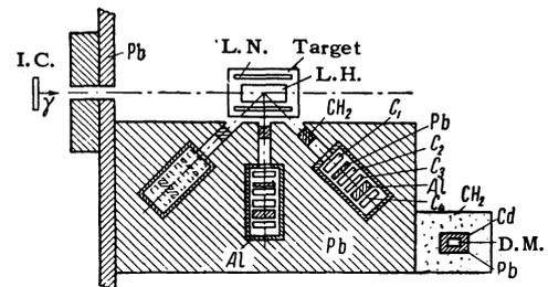
FIG. 1. Schematic diagram of the array. L. H. – Liquid hydrogen, L. N. – liquid nitrogen, I. C. – ionization chamber, D. M. – differential monitor, C<sub>1</sub>, C<sub>2</sub>, C<sub>3</sub>, C<sub>4</sub> – scintillation counters.
