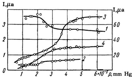
FIG. 4. The current through magnetic slits as a function of hydrogen pressure in the chamber. The number for each curve corresponds to the slit number. The scale at the right refers to Curves 1 and 2; the scale at the left corresponds to Curves 3 and 4.
