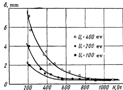
FIG. 6. The effective width of the magnetic slit  $\delta$  as a function of field strength in the slit.
