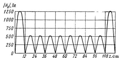
FIG. 2. Magnetic field distribution along the axis of a system;  $H_z$  is the magnetic field at the axis of the chamber.
