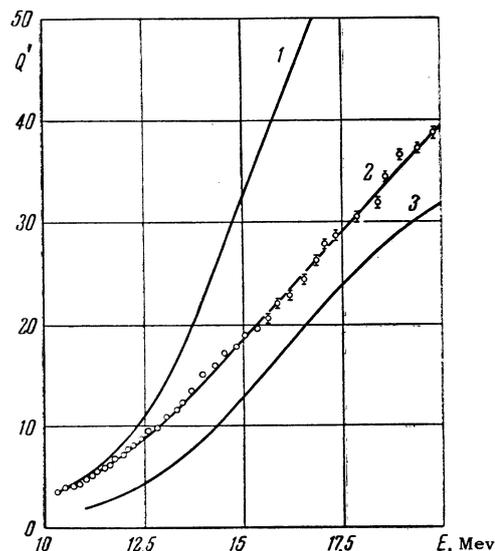
FIG. 2. Photoneutron yield ( $Q'$ ) as a function of the electron-beam energy. To determine the absolute value of the yield (per electron),  $Q'$  must be multiplied by  $10^{-4}$ .
