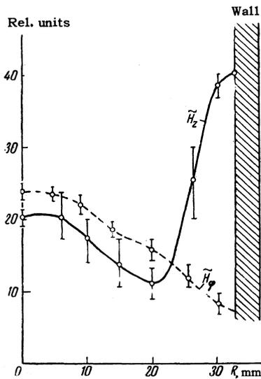
FIG. 9. Radial distribution of the components  $\tilde{H}_z$  and  $\tilde{H}_\phi$  of the amplitude of the high-frequency magnetic field obtained in the arrangement with frequency 50 Mc/sec for  $H_p \sim 800$  oe in hydrogen ( $p = 9 \times 10^{-4}$  mm of mercury).
