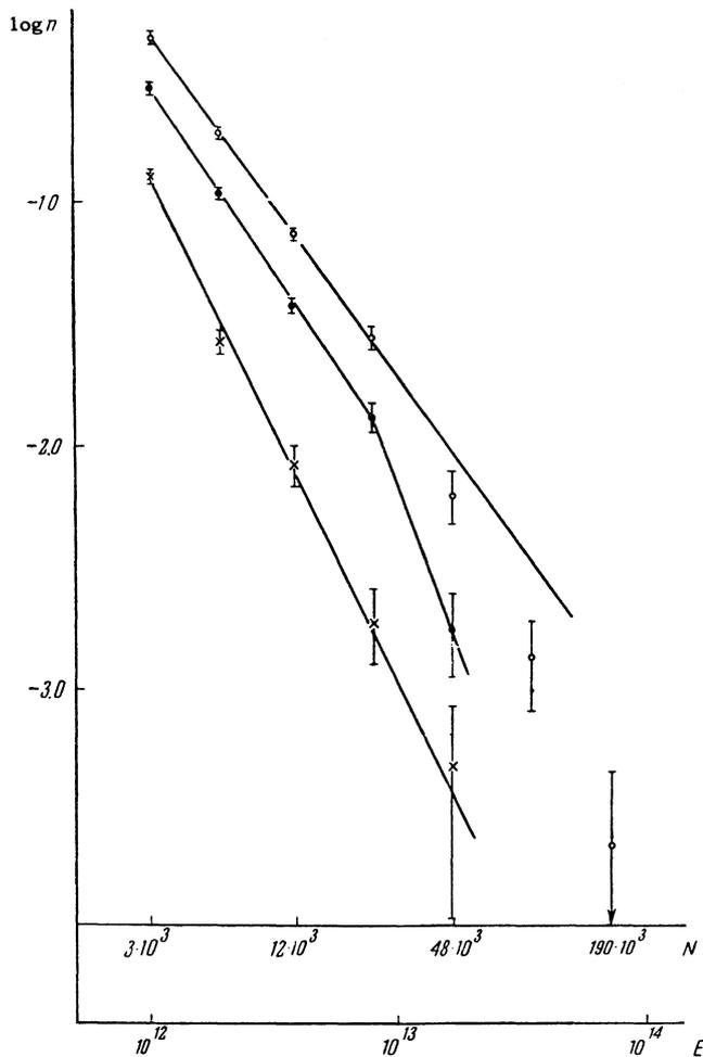
FIG. 3. Integral size distribution of ionization bursts produced by nuclear-active particles (lower scale shows the particle energy):  $\circ$  - all cases;  $\bullet$  - bursts unaccompanied by showers with a number of particles  $\geq 10^5$ ;  $\times$  - ionization bursts unaccompanied by showers with a number of particles  $\geq 6 \times 10^3$ . The y axis represents the flux of nuclear-active particles per  $\text{m}^2$  per hour (logarithmic scale).
