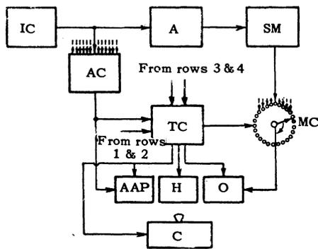
FIG. 2. Block diagram of the electronic circuitry: IC – ionization chamber, A – amplifier, SM – switch and memory cell, AC – addition circuit, TC – trigger and control circuit, AAP – analyzer of added pulses, H – hodoscope, O – oscilloscope, C – camera, MC – mechanical commutator.
