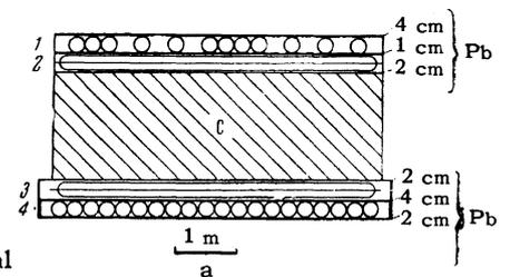
FIG. 1. a - vertical cross section through the detector of nuclear-active particles and high-energy electron-photon showers; b - position of the hodoscope points above the detector.
