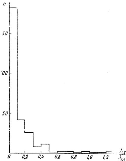
FIG. 2. Distribution of EAS based on the ratio  $J_{1,2}/J_{3,4}$ , (abscissas). The ordinates represent the number of showers with given ratio  $J_{1,2}/J_{3,4}$ .
