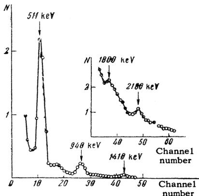
FIG. 5.  $\gamma$  spectrum of Co<sup>55</sup> measured with scintillation  $\gamma$  spectrometer. The hard portion of the  $\gamma$  spectrum, measured with a 25-mm lead filter, is shown in the upper right corner.
