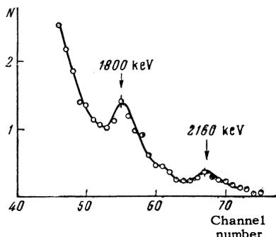
FIG. 12.  $\gamma$  spectrum of V<sup>47</sup>, measured with a lead filter 25 mm thick.
