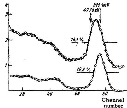
FIG. 6.  $\gamma$  spectrum of Co<sup>55</sup> (upper curve) and  $\gamma$  spectrum of annihilation radiation of Cu<sup>64</sup> (lower curve), measured with conical lead collimator.
