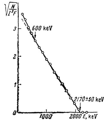
FIG. 9. Fermi plot for  $\beta^+$  spectrum of  $\text{Mn}^{51}$ .
