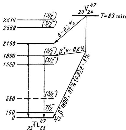
FIG. 13. Decay scheme of V<sup>47</sup>.
