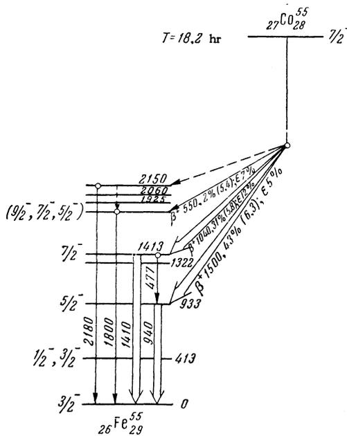
FIG. 8. Decay scheme of  $\text{Co}^{55}$ , from<sup>[7]</sup>.
