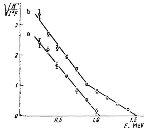
FIG. 7. Fermi plot of coincidences between  $\beta^+$  particles and 1410-keV  $\gamma$  quanta (curve a) or 940-keV  $\gamma$  quanta (curve b) for Co<sup>55</sup>.
