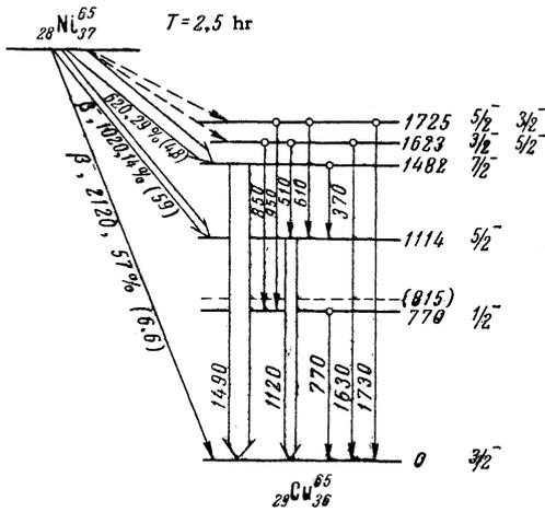
FIG. 4. Level scheme for the decay of Ni<sup>65</sup>, from [4].
