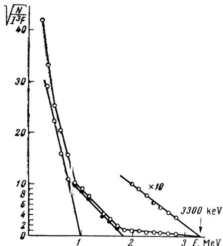
FIG. 14. Fermi plot for  $\beta^-$  spectrum of  $\text{Se}^{83}$ .
