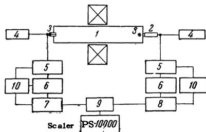
FIG. 1. Block diagram of setup for measuring  $\beta\gamma$  coincidences: 1—magnetic spectrometer, 2—photomultiplier, 3—end-window counter, 4—high-voltage source, 5—cathode follower, 6—amplifier, 7—delay block, 8—differential analyzer, 9—coincidence circuit, 10—rectifier (200 V), S—radio-active source.
