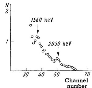
FIG. 10.  $\gamma$  spectrum of  $\text{Mn}^{51}$ , measured with a lead filter 25 mm thick.
