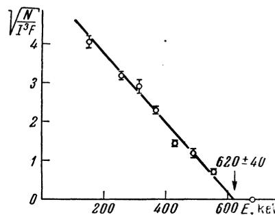
FIG. 2. Fermi plot for the coincidences between  $\beta^-$  particles and 1490-keV  $\gamma$  quanta in  $\text{Ni}^{65}$ .
