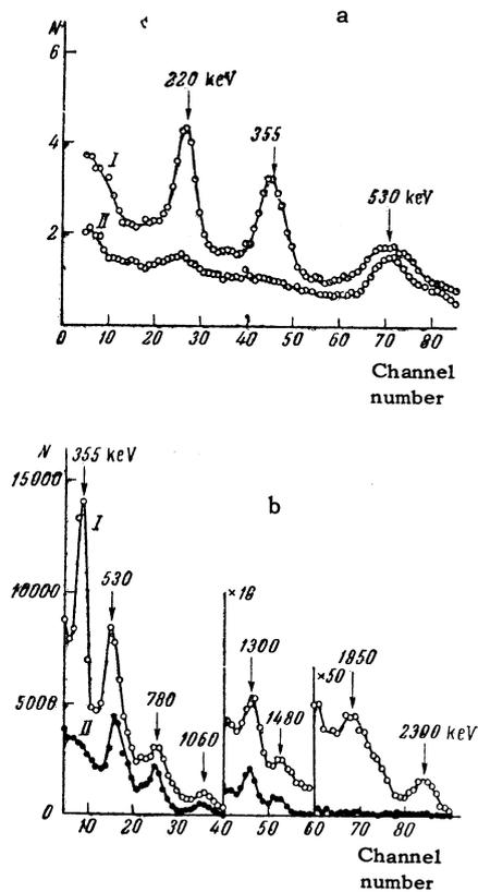
FIG. 15.  $\gamma$  spectrum of  $\text{Se}^{83} + \text{Br}^{82}$ ; a — soft part of the spectrum, b — hard part. Lower curves correspond to the  $\gamma$  spectra measured after several hours.
