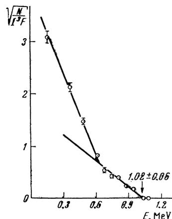
FIG. 3. Fermi plot for the spectrum of coincidences between  $\beta^-$  particles and  $\gamma$  quanta with energy  $E_\gamma \geq 1120$  keV in  $\text{Ni}^{65}$ .
