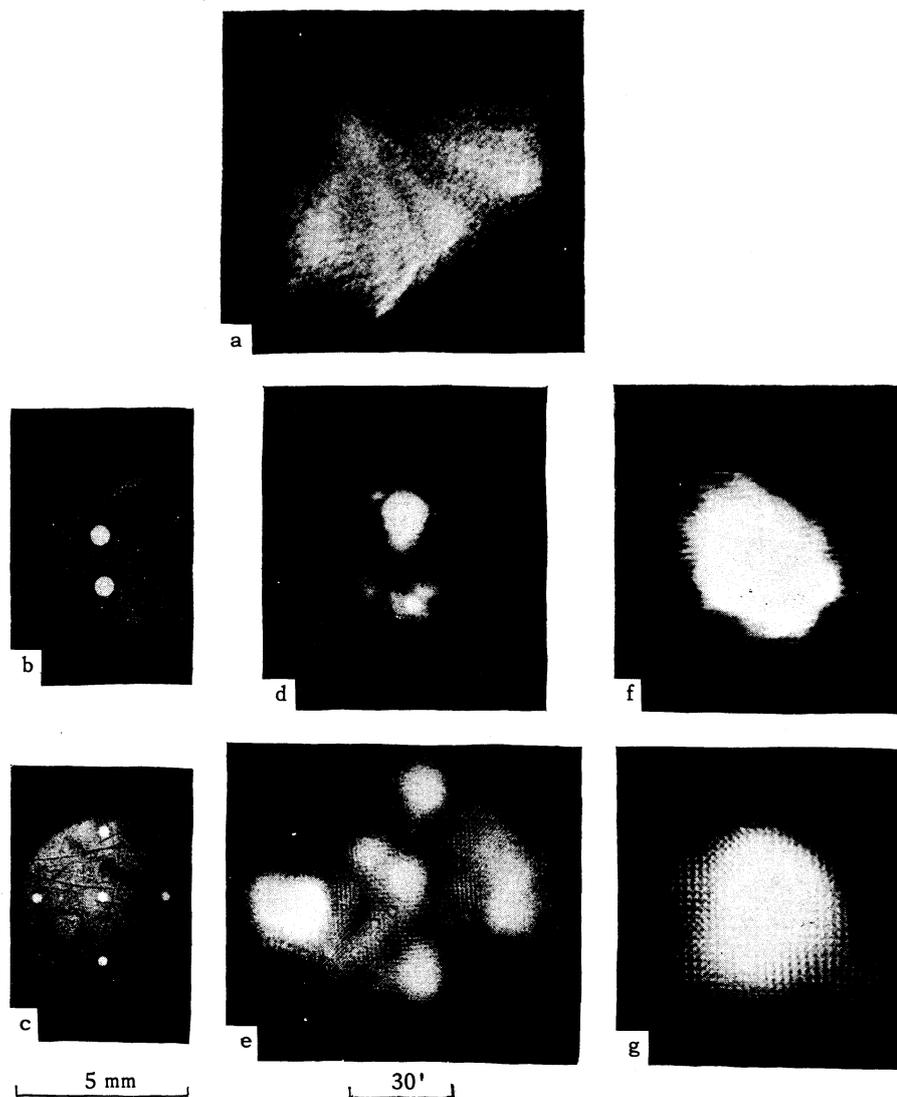
FIG. 3. a—pattern in plane F without diaphragm D; b—configuration of the two-hole diaphragm with respect to the image of the end face of the crystal; c—the same for the five-hole diaphragm; d, e—pattern in plane F for the two-hole and five-hole diaphragms, respectively; f, g—pattern in plane  $F_1$  for the two-hole and five-hole diaphragms, respectively.
