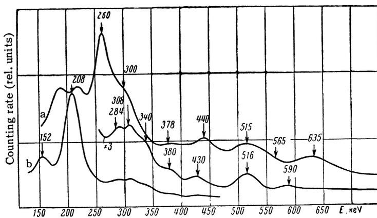
FIG. 2. Spectra of coincidence with (a) 80-keV  $\gamma$  rays [using NaI(Tl) crystal 40 mm high], and (b) 117-keV  $\gamma$  rays [using NaI(Tl) crystal 10 mm high].
