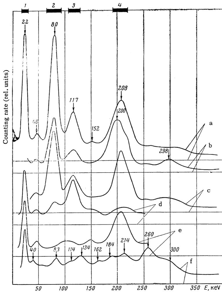
FIG. 1. Typical spectra of  $\gamma$  rays from  $\text{Ag}^{108}$ . a – single-crystal spectrum of  $\gamma$  rays absorbed in a filter consisting of 1 mm Pb, 0.5 mm Sn, and 0.1 mm Zn. Coincidence spectra discriminated in control channel: b, c – hard  $\gamma$  rays close to the neutron binding energy; d – region 4; e – region 3; f – region 2.
