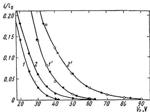
FIG. 2. High-energy part of the current-voltage retardation curves of scattered  $\text{Cs}^+$  ions (1,  $U = 150$  eV; 2,  $U = 250$  eV) and Rb ions ( $1'$ ,  $U = 150$  eV;  $2'$ ,  $U = 250$  eV, open circles). The black dots on curves  $1'$  and  $2'$  were obtained from the points on curves 1 and 2 by increasing the abscissa scale by factors of 1.50 and 1.67 respectively.
