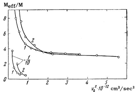
FIG. 1. Dependence of the ratio  $M_{eff}/M$  on the square of the incident-ion velocity: 1)  $Cs^+$ , 2)  $Rb^+$ .
