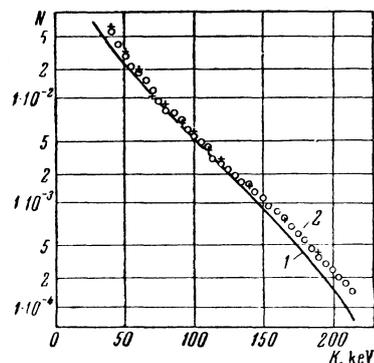
Internal bremsstrahlung spectrum accompanying the beta decay of  $Ca^{45}$ : 1 – curve calculated from the theory of Knipp and Uhlenbeck ( $Z = 0$ ); 2 – experimental points (o – initial measurements, + – control measurements).
