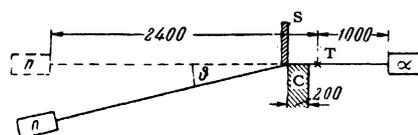
FIG. 1. Diagram of the experiment: T - target, S - scatterer, C - collimator, n and α - neutron and alpha-particle detectors (the dimensions are in millimeters).
