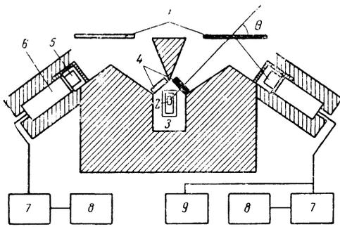
FIG. 2. Experimental setup under the "plane" geometry conditions: 1) scatterers; 2) source; 3) electrical furnace; 4) Fe and Cd absorbers (in the self-absorption experiment); 5) NaI:Tl crystal; 6) FÉU-12B; 7) single-channel pulse analyzer; 8) PS-10 000 scaler; 9) 100-channel pulse analyzer AN-100.
