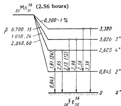
FIG. 1.  $Mn^{56} \rightarrow Fe^{56}$  decay scheme including cascades leading to the 0.845 MeV level (energies are given in MeV).
