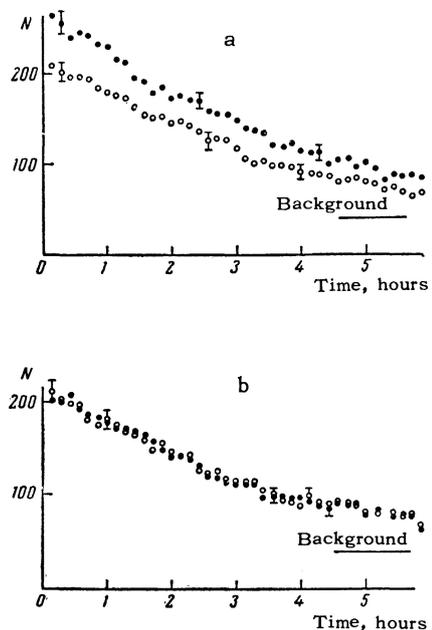
FIG. 4. Intensities of resonant scattering of  $\gamma$ -quanta on Fe<sup>56</sup> nuclei ("plane" geometry): a) gaseous source; b) solid source; ● – Fe scatterer; ○ – Cu scatterer. The ordinate axis gives the number of counts per 2 min.
