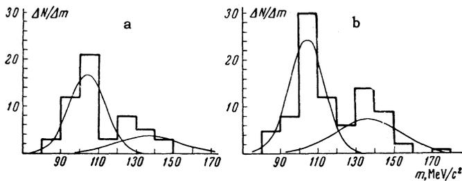
FIG. 1. Mass spectra of stopping mesons. a – experiment I [ $\epsilon(\text{He}^4) = 4.9\%$ ], b – II [ $\epsilon(\text{He}^3) = 14.3\%$ ]. The smooth lines are resolving power curves.
