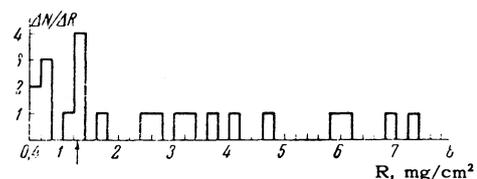
FIG. 2. Measured spectrum of secondary particle ranges in experiment II [ $\epsilon(\text{He}^3) = 14.3\%$ ]. The arrow indicates the predicted tritium range in the reaction  $\mu^- + \text{He}^3 \rightarrow \text{H}^3 + \nu$ .
