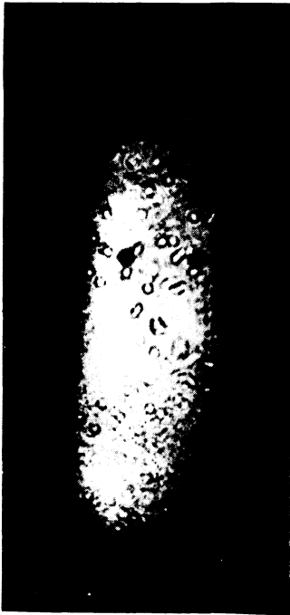
FIG. 3. Photograph of the cross section of a second harmonic beam excited by an unfocused ruby laser beam in a KDP crystal 1 cm long.
