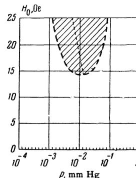
FIG. 9. The region in which the anomalous field penetration into the plasma is observed ( $f = 5.6$  Mc/sec).
