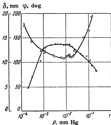
FIG. 6. The phase shift of the oscillating field at the axis and the plasma edge and the skin depth as functions of the Xe pressure: ●— $\varphi = f(p)$ , ○— $\delta = f(p)$ ;  $f = 0.9$  Mc/sec,  $H_0 = 42$  Oe.
