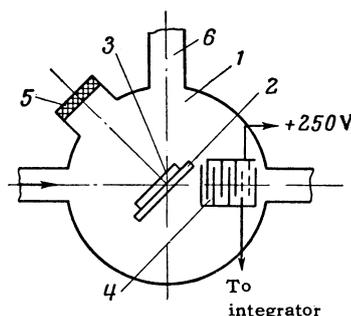
FIG. 1. Schematic representation of the experimental setup: 1) vacuum chamber; 2) target support; 3) zinc sulfide screen; 4) secondary-emission monitor; 5) window for observing the beam image on the screen; 6) light guide. The arrow on the right shows the direction of the electron beam.
