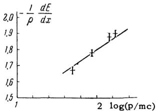
FIG. 5. Theoretical curve and experimental values (+) of the electron energy losses in a polystyrene film  $10^{-5}$  cm thick.
