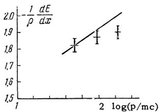
FIG. 7. Theoretical curve and experimental values (+) of the electron energy losses in a polystyrene film  $2 \times 10^{-4}$  cm thick.
