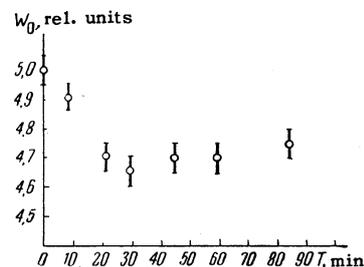
FIG. 4. Dependence of the specific scintillation of a film on the duration of irradiation.
