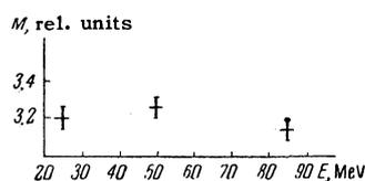
FIG. 2. Dependence of the secondary-emission monitor efficiency on the electron energy.
