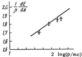
FIG. 6. Theoretical curve and experimental values (+) of the electron energy losses in a polystyrene film  $2 \times 10^{-5}$  cm thick.
