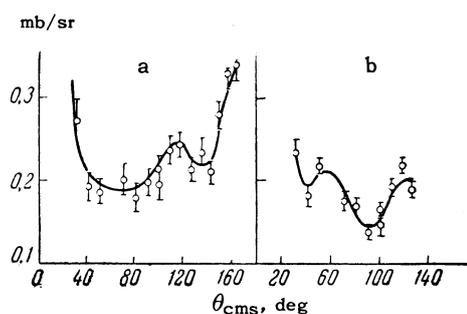
FIG. 1. Angular distribution of alpha particles in the  $B^{11}(d, \alpha)Be^9$  reaction for the ground (a) and second excited (b) states of  $Be^9$ ;  $E_d = 6.6$  MeV.
