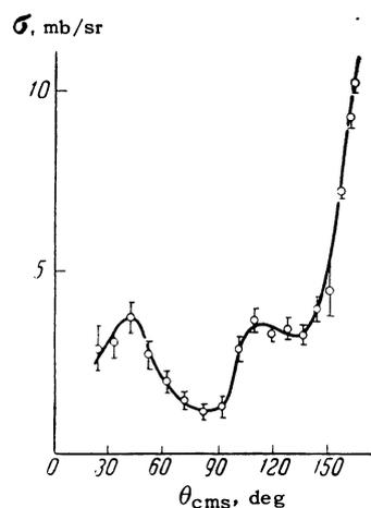
FIG. 2. Angular distribution of  $O^{16}(d, \alpha)N^{14}$  reaction for the second excited (3.94 MeV) state;  $E_d = 6.6$  MeV.
