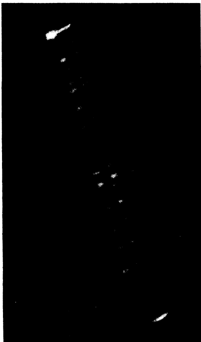
FIG. 5. Photograph of a particle track in a neon-filled streamer chamber ( p = 1 atm, E = 8 kV/cm), obtained with a long rise time of the high voltage pulse.
