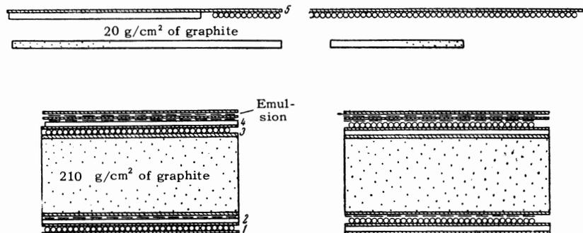
FIG. 1. Diagram of array in two projections: 1–5) rows of ionization chambers (area of array 10 m<sup>2</sup>)
