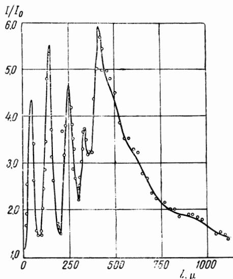
FIG. 6. Distribution of luminescence intensity through the depth of the sample during generation.
