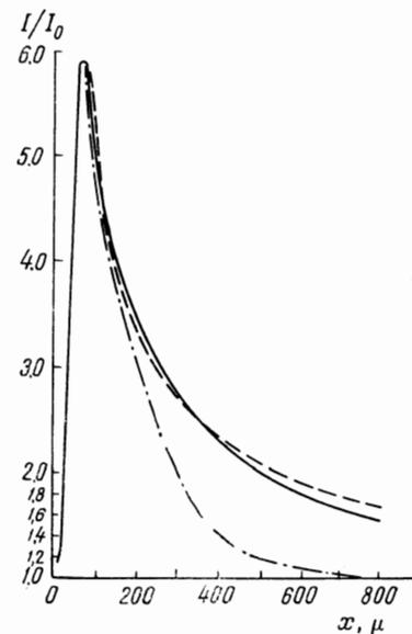
FIG. 5. Distribution of the intensity of recombination radiation at exciting-radiation power below the threshold of self-excitation: dashed — theoretical curve calculated by formula (10) at  $K_0^{(2)} = 63 \text{ cm}^{-1}$  ( $I_0 = 7 \text{ MW/cm}^2$ ) solid curve — experimental relation; dash-dot curve — theoretical curve for single-photon absorption ( $n = 1$ ).
