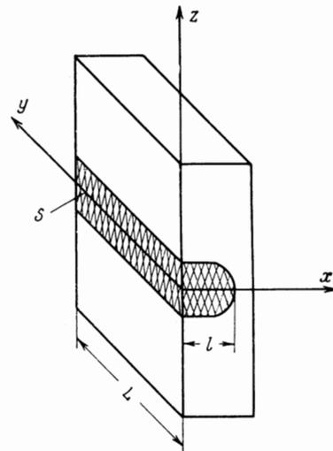
FIG. 4.  $S$  — area of irradiated semiconductor surface,  $l$  — depth of penetration of exciting radiation,  $L$  — distance between the sample faces that form the resonator.
