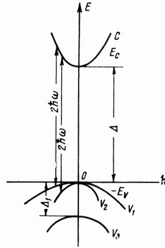
FIG. 1. Band structure of GaAs.  $C$  – conduction band,  $V_1, V_2, V_3$  – valence bands,  $\Delta$  – width of forbidden band. The arrows denote the transitions of electrons from the valence band to the conduction band, accompanied by absorption of two quanta of pump light. The energy is reckoned from the “ceiling” of the valence bands  $V_1$  and  $V_2$ .
