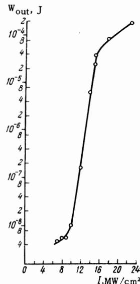
FIG. 7. Dependence of the energy  $W$  of the generated light pulse on the density of the exciting light flux  $I$ . The energy of the exciting light pulse is constant at  $0.07 \text{ J}$ .
