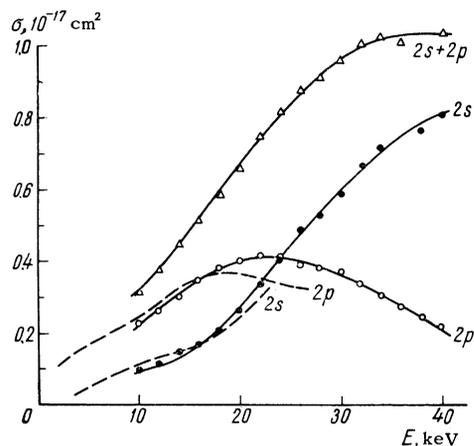
FIG. 4. Cross sections for the excitation of the 2s and 2p states and their sum for the process of the charge exchange of protons in helium, plotted as a function of the proton energy: ● — cross sections for the excitation of the 2s state; ○ — cross sections for the excitation of the 2p state; △ — sum of the excitation cross sections for the 2s and 2p states; dashed curves give the excitation cross sections of the 2s and 2p states reported in [7, 14].
