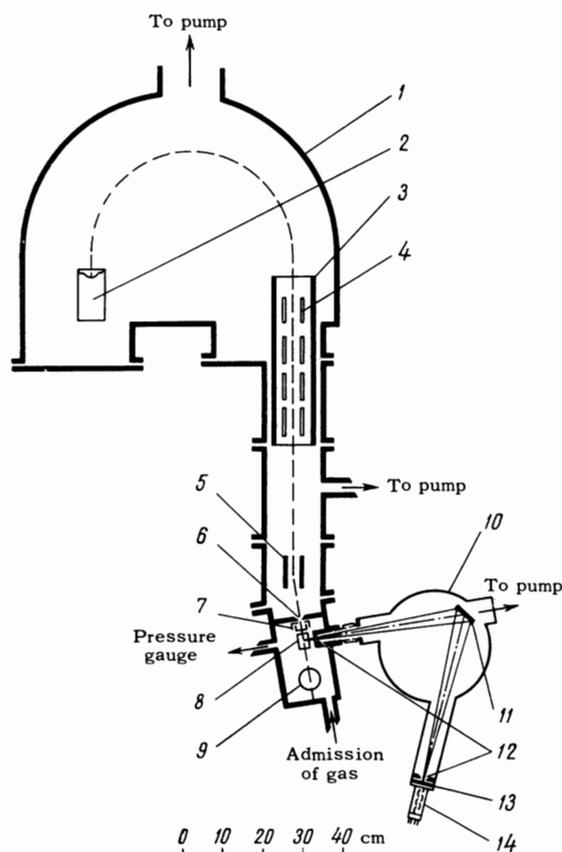
FIG. 1. Schematic diagram of the apparatus: 1) vacuum chamber of the mass spectrometer; 2) ion source; 3) magnetic screen; 4) electrodes of quadrupole lenses; 5) deflecting capacitor; 6) entry slit of the collision chamber; 7) extensible ion detector; 8) capacitor producing the de-exciting electric field; 9) trap; 10) vacuum monochromator; 11) bent diffraction grating; 12) entry and exit slits of the vacuum monochromator; 13) screen covered with sodium salicylate; 14) photomultiplier.
