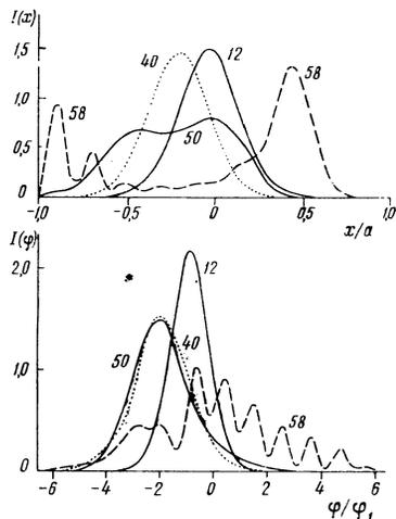
FIG. 6. The same as in Fig. 2, but for the case when the index of refraction of the medium in the resonator has an inhomogeneity of the wedge type.
