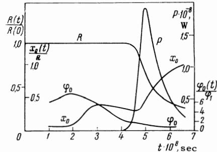
FIG. 1. Variation in the power  $P(t)$  of a giant light pulse, the total number of active particles in the resonator  $R(t)$ , the half-width of the region of generation at half-height  $x_0(t)$ , the half-divergence of the radiation at half-height  $\varphi_0(t)$  in the case that the index of refraction of the medium in the resonator has an inhomogeneity of the positive lens type.
