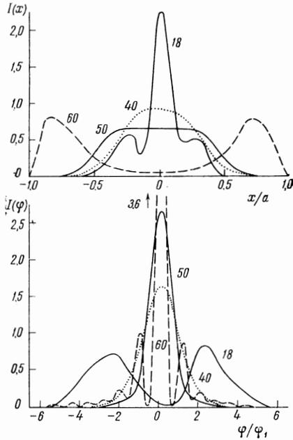
FIG. 2. Instantaneous distributions of intensity over the end  $I(x)$  and with respect to the angles  $I(\varphi)$  ( $a$  is the half-width of the resonator,  $2\varphi_1$  is the divergence with respect to the half-height of the principal type of oscillations) when the index of refraction of the medium in the resonator has an inhomogeneity of the positive lens type (numbers adjacent to the curves represent time in nsec).
