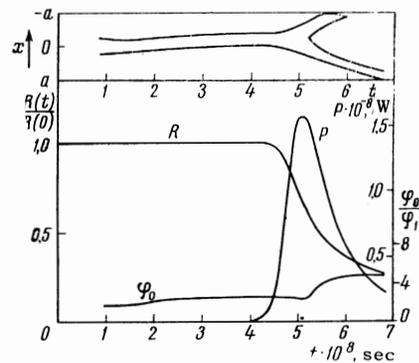
FIG. 5. The same as in Fig. 1, but for the case when the index of refraction of the medium in the resonator has an inhomogeneity of the wedge type. At the top is shown the motion of the field distribution along the end of the generator (solid lines correspond to the half-maxima of the distribution.)
