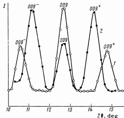
FIG. 5. Neutron-diffraction patterns of  $(\text{Sr}_{0.8}\text{Ba}_{0.2})_2\text{Zn}_2\text{Y}$  in the region of the 009 reflection at 293°K. The neutron wavelength was 1.70 Å. 1)  $H = 3000$  Oe,  $H \perp \epsilon$ ; 2)  $H = 0$ .
