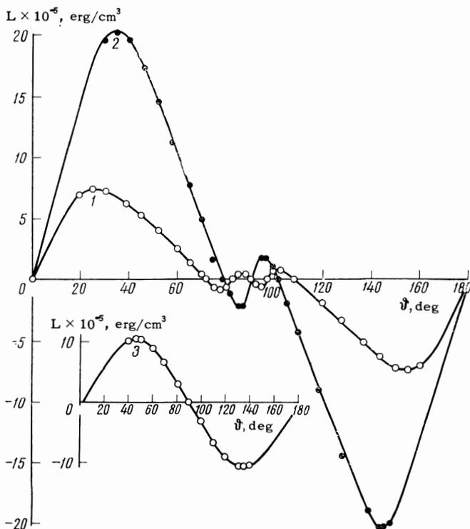
FIG. 2. Torque curves of  $(\text{Sr}_{0.8}\text{Ba}_{0.2})_2\text{Zn}_2\text{Y}$ : 1) at 293°K, 2) at 77°K, and the torque curve of  $\text{Ba}_2\text{Zn}_2\text{Y}$  at 293°K (3).
