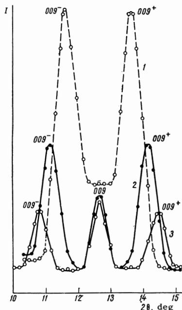
FIG. 4. Neutron-diffraction patterns of  $(\text{Sr}_{0.8}\text{Ba}_{0.2})_2\text{Zn}_2\text{Y}$  in the region of the 009 reflection (1 denotes the number of pulses per minute, in relative units;  $\theta$  is the Bragg angle). The neutron wavelength was 1.07 Å. 1) 4.2°K; 2) 293°K; 3) 370°K.
