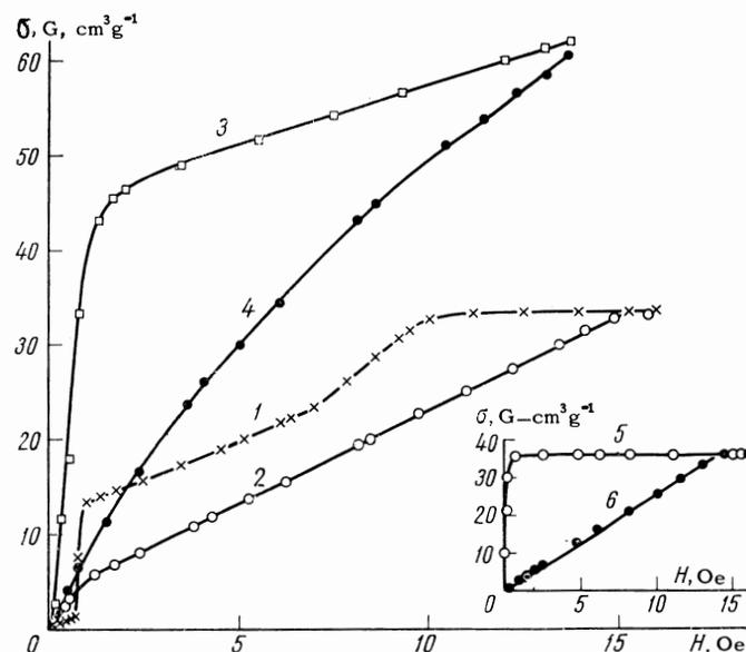
FIG. 1. Magnetization curves of  $(\text{Sr}_{0.8}\text{Ba}_{0.2})_2\text{Zn}_2\text{Y}$ : 1)  $H \perp c$  at 293°K; 2)  $H \parallel c$  at 293°K; 3)  $H \perp c$  at 77°K; 4)  $H \parallel c$  at 77°K; magnetization curves of  $\text{Ba}_2\text{Zn}_2\text{Y}$  at 293°K: 5)  $H \perp c$ ; 6)  $H \parallel c$ .
