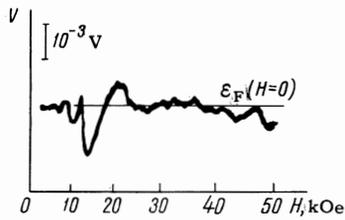
FIG. 1. Shift of Fermi level in a magnetic field. The magnetic field is parallel to the bisector axis of the bismuth single crystal. The scale along the V axis is for the oscillating component of the Fermi level.
