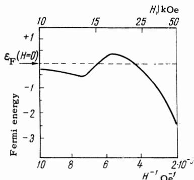
FIG. 4. Monotonic component of the Fermi level in a magnetic field. Magnetic field parallel to the binary axis.
