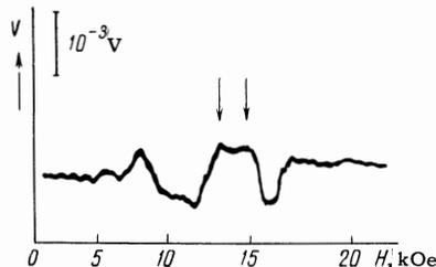
FIG. 5. Oscillations of Fermi level in a magnetic field. Magnetic field parallel to the binary axis. The arrows indicate the spin splitting.
