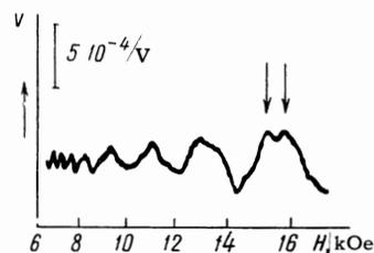
FIG. 6. Oscillations of Fermi level in a magnetic field. Magnetic field parallel to the trigonal axis. The arrows indicate the spin splitting.
