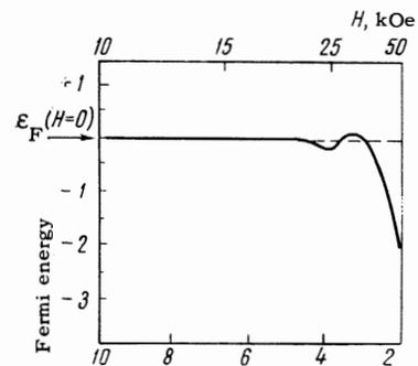
FIG. 3. Monotonic component of the Fermi level (MeV) in a magnetic field. Magnetic field parallel to the bisector axis.
