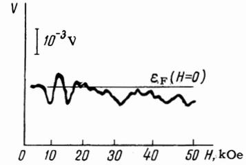
FIG. 2. Shift of Fermi level in a magnetic field. The magnetic field is parallel to the binary axis of the single-crystal bismuth. Scale along the V axis is for the oscillating component of the Fermi level.
