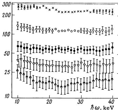
FIG. 8. Ratio of the yield of resonance radiation for different numbers of layers  $n$  to the yield for  $n = 300$ :  $\times$  -  $n = 200$ ,  $\circ$  - 100,  $\bullet$  - 50,  $\nabla$  - 25,  $\circ$  - 10. The ordinate represents the relative yield of radiation, expressed in units of number of layers.
