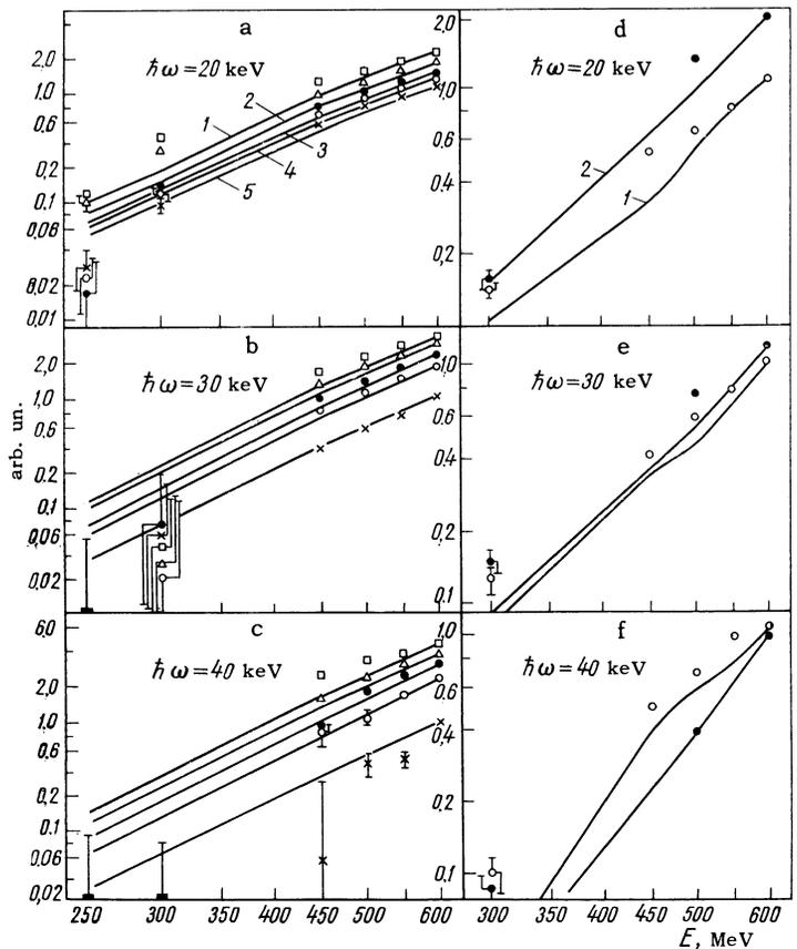
for different layered media is shown in Fig. 7. The data are given in arbitrary units. In these plots the theoretical curves are normalized to the experimental data at the point  $E = 600$  MeV. In the region of comparatively low electron energies a stronger dependence of intensity on electron energy is observed than is expected from theory. Over the entire energy region studied from 250 to 600 MeV this dependence has a form  $\sim E^\gamma$ , where  $\gamma \gtrsim 2$ .
