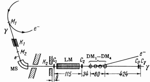
FIG. 1. Sketch of the experimental setup:  $M_1, M_2$  – internal and external targets,  $K_1, K_2$  – collimators, MS – magnetic spectrometer, LM – layered medium,  $DM_1$ – $DM_4$  – deflecting magnets,  $C_1, C_2, C_3$  – scintillation counters,  $C_4$  –  $\gamma$  spectrometer. Also shown are certain linear dimensions in centimeters.
