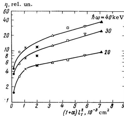
FIG. 9. The ratio ( $\eta$ ) of the experimental yield of resonance radiation to the resonance radiation obtained from theory with inclusion of absorption, as a function of the quantity  $(1 + \alpha)l_1^2$  for different layered media. The parameters of the layered media are as follows:
