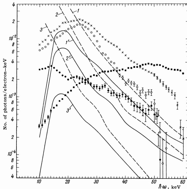
FIG. 5. Differential spectrum of resonance radiation in a layered medium with  $l_1 = 2.83 \times 10^{-3}$  cm,  $\alpha = 18.8$ ;  $n = 1050$ . Curves 1-3 - theory of resonance radiation without inclusion of absorption, curves 1'-3' - with inclusion of absorption. Electron energy (in MeV):  $\times$ , 1,1' - 600;  $o$ , 2,2' - 500;  $\bullet$ , 3,3' - 300;  $\blacksquare$  - bremsstrahlung spectrum.
