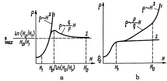
Dependence of the resistance on the intensity of the magnetic field in metals with closed Fermi surfaces: a – number of electrons and holes compensated ( $n_1 = n_2$ ) b – number of electrons not equal to the number of holes ( $n_1 \neq n_2$ ). Curves 1 – for  $\alpha \neq \pi/2$ , curves 2 – for  $\alpha = \pi/2$ .
