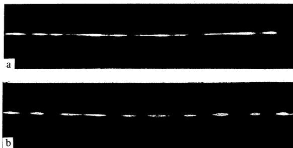
Fig. 1. Oscillograms of light spikes taken from the EOC screen: a—hf generator disconnected; b—hf generator turned on, frequency  $f = 680$  MHz. Injection current  $I = 1.2I_{\text{thr}}$  in both cases. Oscillogram sweep duration  $\approx 14$  nsec.
