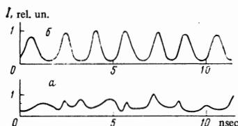
Fig. 2. Results of photometry of the oscillogram of the solid-state laser emission: a—hf generator off; b—solid-state laser emission in the synchronization mode.
