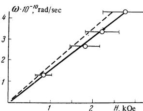
FIG. 4. Maximum frequency of radiation from a plasma vs. magnetic field. Dashed line— $\omega_{H^e} = eH/mc$ .
