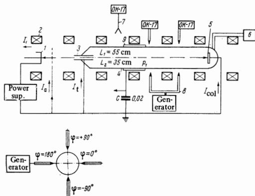
FIG. 1. Diagram of setup: 1—cathode, 2—magnetic-field coils, 3—pressure reducing tube, 4—glass chamber, 5—collector, 6—mechanical leak valve, 7—horn antenna, 8—antennas for  $\lambda = 8$  mm radiation, 9—metallic cylinder for measurement of the charge oscillations ( $l = 10$  cm).
