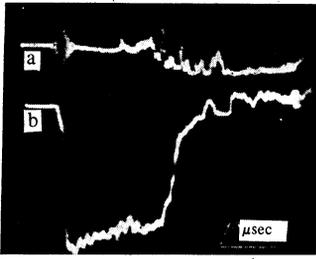
FIG. 8. Intensity of microwave radiation ( $\lambda = 14$  cm) passing through the plasma: a—downward beam deflection corresponds to a decrease in the intensity of the received signal. Positive pips—radiation of plasma proper; b—collector current.  $U_0 = 10$  kV,  $I_{col} = 6.5$  A,  $H = 800$  Oe,  $P_1 = 10^{-4}$  mm Hg.
