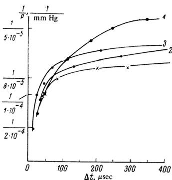
FIG. 3. Plot of  $1/P_1$  vs. duration of the stable stage  $\Delta t$ .  $L_2 = 35 \text{ cm}$ . Curve 1— $I = 2 \text{ A}$ ,  $H = 3 \text{ kOe}$ ; 2— $I = 2 \text{ A}$ ,  $H = 1.5 \text{ kOe}$ ; 3— $I = 3.7 \text{ A}$ ,  $H = 1.5 \text{ kOe}$ ; 4— $I = 10 \text{ A}$ ,  $H = 1.5 \text{ kOe}$  and  $H = 3 \text{ kOe}$ .
