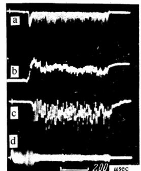
FIG. 2.  $U_0 = 10$  kV,  $I_{col} = 10$  A,  $H = 1500$  Oe,  $P_1 = 7.5 \times 10^{-5}$  mm Hg: a—microwave radiation from plasma; b—collector current; c—intensity of  $\lambda = 8$  mm radiation passing through the plasma (downward deflection of the beam means decrease of the radiation transmitted through the plasma); d—oscillations of the charge of a plasma-cylinder section of length  $l = 10$  cm.
