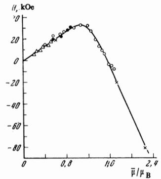
FIG. 4. Dependence of the average field  $\bar{H}$  at the nuclei of impurity  $\text{Sn}^{119}$  atoms in metallic ferromagnets on the magnitude of the average magnetic moment  $\bar{\mu}$  per atom of the alloy:  $\circ$  — CoPd,  $\bullet$  — FePd,  $\Delta$  — CuNi,  $\times$  — Fe, Co, Ni.
