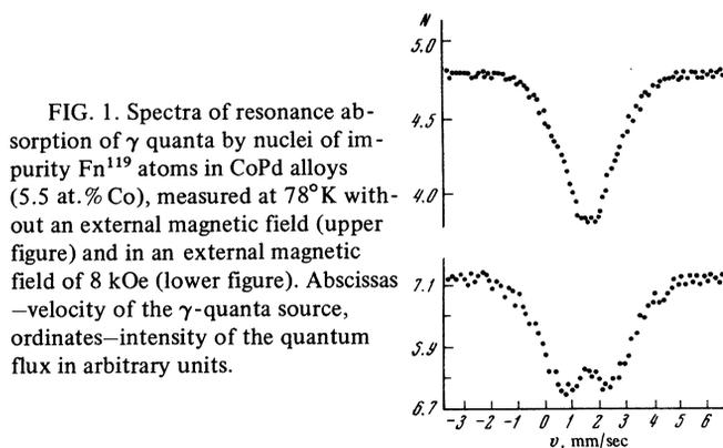
FIG. 1. Spectra of resonance absorption of  $\gamma$  quanta by nuclei of impurity  $\text{Sn}^{119}$  atoms in CoPd alloys (5.5 at.% Co), measured at 78°K without an external magnetic field (upper figure) and in an external magnetic field of 8 kOe (lower figure). Abscissas—velocity of the  $\gamma$ -quanta source, ordinates—intensity of the quantum flux in arbitrary units.
