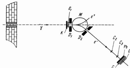
FIG. 1. Experimental arrangement.  $\gamma$  — beam of  $\gamma$  rays; K — lead converter; M — magnet;  $D_1$  and  $D_2$  — lead diaphragms;  $C_1$ ,  $C_2$ ,  $C_3$  — scintillation counters which distinguish the electron beam  $e^-$ ;  $C_4$  scintillation counter spectrometer; Pb — lead absorber; C — graphite absorber.
