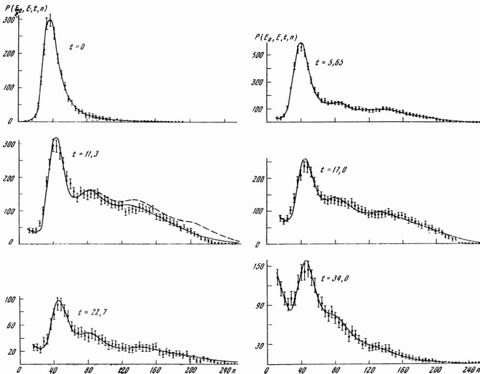
FIG. 2. Pulse height distributions  $P(E_0, E, t, n)$  from counter  $C_4$  for  $E_0 = 217$  MeV,  $t_C = 0$  ( $E = 2$  MeV); the dashed line shows the spectrum measured for the case when an additional lead block is placed beyond counter  $C_4$  (backscattering of shower particles). The curves represent Eq. (2) calculated by the method of least squares. Values of  $t$  (in g/cm<sup>2</sup> Pb) are indicated in the figure. The analyzer counting rates shown are summed in groups of four channels.
