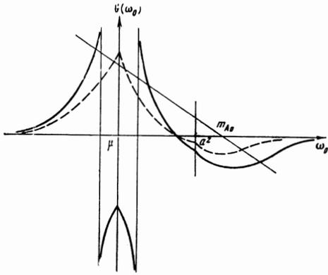
FIG. 3. Behavior of the function  $G(\omega_0)$ . For small values of  $\gamma_{02}$ ,  $G(\omega_0)$  does not have any poles (the dotted curve). Starting at  $\gamma_{02} = \gamma'_{02}$  two poles appear at the point  $\omega_0 = \mu$ , moving away from this point in opposite directions as the value of  $\gamma_{02}$  increases.
