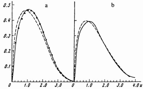
FIG. 2. Comparison of the various approximations for the electron distribution function: a)  $n = -1$ ,  $\gamma = 0.1$ ; dotted — the function  $\sqrt{u} f_0^{(1)}$ ; solid line — solution of Eq. (9) in the next approximation; points — the function  $\sqrt{u} f_0^{(2)}$ ; b)  $n = 0$ ,  $\gamma = 1$ ; dotted —  $\sqrt{u} f_0^{(1)}$ ; solid line — solution of Eq. (9) in the next approximation.
