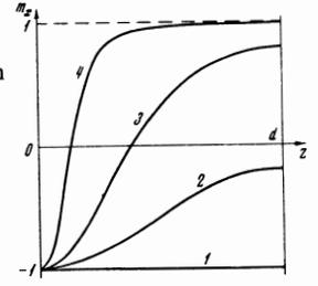
FIG. 2. Distribution of magnetization over the film thickness. Curve 1 ( $k^2 = 0$ ) corresponds to  $H_0 < H_u$ , curves 2 ( $k^2 = 0.4$ ), 3 ( $k^2 = 0.9$ ), and 4 ( $k^2 = 1 - 10^{-5}$ ) correspond to a sequence of increasing fields at  $H_0 > H_u$ .
