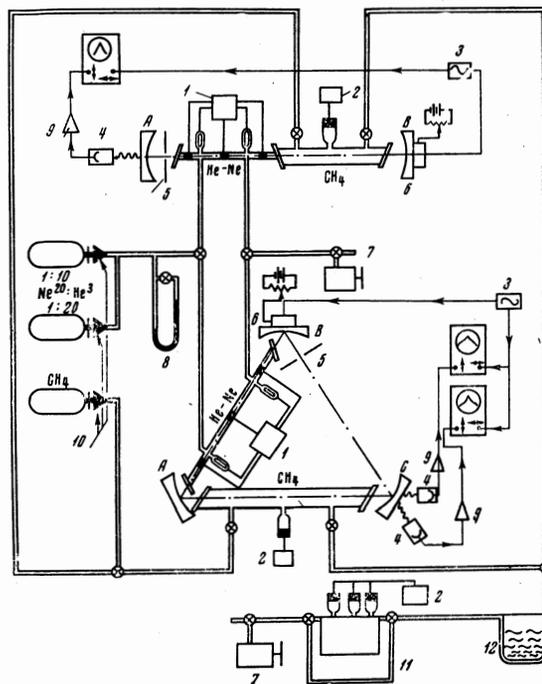
FIG. 4. Experimental setup: 1—power supply, 2—vacuum meter, 3—generator ( $f = 50$  Hz), 4—Ge-Au receiver, 5—diaphragm, 6—piezoceramic, 7—forevacuum pump, 8—oil manometer, 9—amplifier, 10—reductor, 11—diffusion pump, 12—nitrogen trap, A, B, C—flat mirrors.
