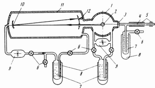
FIG. 1. Schematic diagram of the apparatus: 1) plasma unit resonator; 2) filamentary discharge; 3) lithium fluoride window; 4) low-pressure discharge tube with electrodes; 5, 6) valves; 7) zeolite traps; 8) dewars with liquid nitrogen; 9) fans of the EV50/100 type; 10) diffraction grating; 11) spectrograph; 12) radiation detector. The arrows show the beam path.
