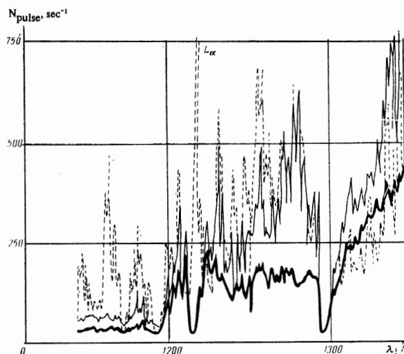
FIG. 3. Spectrum of deuterium plasma (thick curve) recorded with an SFM-3 counter. Power input 9.3 kW; pressure 1 atm; resolution 1 Å. The dashed curve is the spectrum of a low-pressure discharge in hydrogen, and the thin curve is the spectrum of a plasma and a low-pressure discharge.
