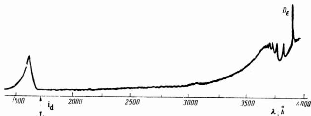
FIG. 2. Spectrum of deuterium plasma recorded with a photomultiplier. Power input 6.6 kW; pressure 1.3 atm; resolution 4 Å ( $i_d$  is the dark current). A quartz filter was used to remove the second-order spectrum in the  $\lambda > 2000\text{Å}$  range. The dip at  $\lambda = 3850\text{Å}$  was due to a minimum in the transfer function of the VM-1 monochromator.
