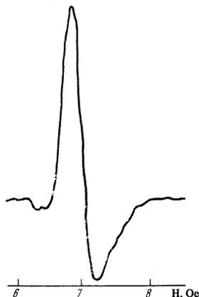
FIG. 5. Signal obtained with a cell 60 cm long ( $\text{Xe}^{136}$ ,  $\lambda = 5.57\mu$ ,  $f = 26.4$  MHz). The registration time constant is 10 sec.
