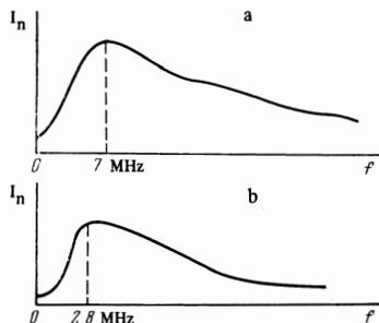
FIG. 4. Noise power spectrum of discharge in  $\text{Xe}^{136}$ : a—maximum light intensity; b—minimum intensity registered by the receiver.
