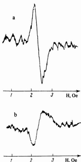
FIG. 3. Inversion of signal on going from an amplifying medium (a) to an absorbing one (b) ( $\text{Xe}^{136}$ ,  $\lambda = 5.57\mu$ ,  $f = 9.1$  MHz).
