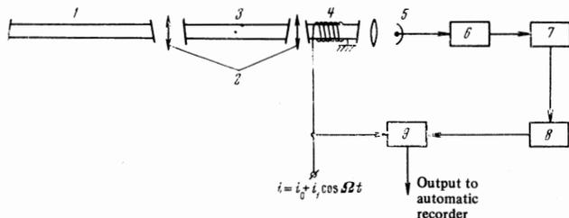
FIG. 1. Block diagram of experimental setup. 1—radiation source, 2—polarizers crossed at an angle  $45^\circ$ , 3—Faraday cell, 4—investigated cell, 5—infrared receiver, 6—tuned amplifier, 7—detector, 8—low-frequency amplifier, 9—synchronous detector.
