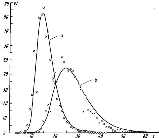
FIG. 5. Distribution of transient time in a laser with NRA at different values of  $\alpha$ ,  $\beta$ ,  $\gamma$ , and  $t_m$ . Solid curve—theory, points—experiment.
