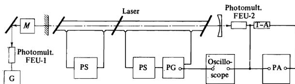
FIG. 1. Diagram of experimental setup. PS—power supply, PG—pulse generator, M—monochromator, G—Galvanometer, T-A—time-amplitude converter, PA—pulse analyzer.
