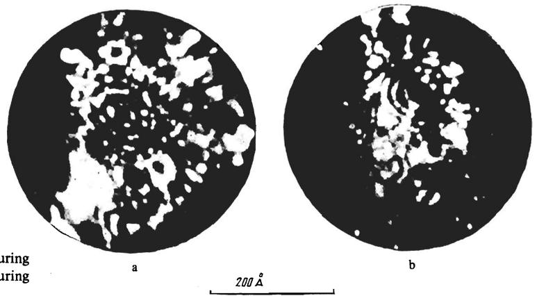
FIG. 3. a—Field ion microgram of a section of an alloy measuring  $\sim 300\text{\AA}$ , containing  $\sim 96.3\%$  Nb. b—Microgram of a section measuring  $\sim 300\text{\AA}$  of the surface of Nb 99.2% pure.
