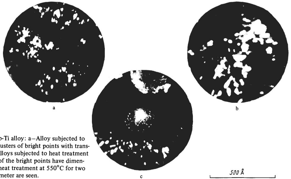
FIG. 1. Field-ion microgram of Nb-Ti alloy: a—Alloy subjected to deep deformation in the cold state. Clusters of bright points with transverse dimensions  $\sim 10\text{Å}$  are seen. b—Alloys subjected to heat treatment at  $400^\circ\text{C}$  for two hours. The clusters of the bright points have dimensions  $20\text{--}50\text{Å}$ . c—Alloy subjected to heat treatment at  $550^\circ\text{C}$  for two hours. Individual zones of  $\sim 300\text{Å}$  diameter are seen.
