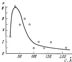
FIG. 2. Distribution of the dimensions of the brightly emitting sections of an alloy subjected to heat treatment (two hours) at  $400^\circ\text{C}$ .
